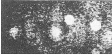
Fig. 3 A reconstructed portion of a double pulsed hologram. The in-focus bubble pair, outside the core, represents a bubble moving at 3.3 m/s. The out-of-focus bubble pair to the right, in the core, reveals a velocity of 5.1 m/s. Re = 5.2 \times 10^5 , x/c = 2 , \alpha = 10 deg.
